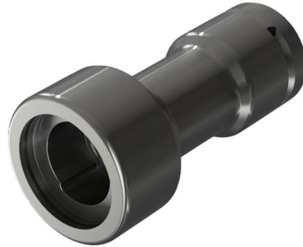
The AutoGRIPPER stud extractor saves time and expense associated with the removal of stud bolts from threaded holes. The extractor is attached to an air impact wrench, installed over the exposed stud, and removes the stud from the hole in seconds. With the AutoGRIPPER, it is possible to immediately identify if a stud can be removed by rotation.
