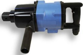
**AIW3300** 1-1/2" drive air impact wrench is a single person operated tool delivering 3,300 ft-lb. working torque and a maximum torque of 4,000 ft-lb. Twin hammer mechanisms and a 7 vane motor deliver high output. Bronze end plates increase motor durability. Includes an integral muffler for noise reduction, built-in lubricator, and a 3-piece housing for easy repair.
